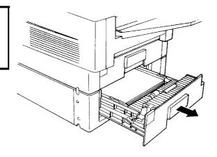
2. Clean the paper feed roller [U] with the soft damp cloth, while rotating it in the direction shown in the diagram.
